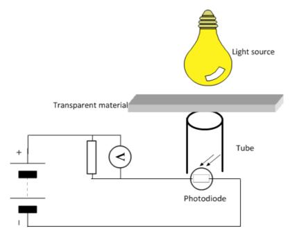
The following results were obtained when various materials were placed in turn across the top of the photodiode tube.
