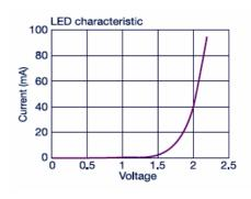
3.10.4 Explain how a resistor connected in series with the LED can limit the power that is consumed by the LED.
