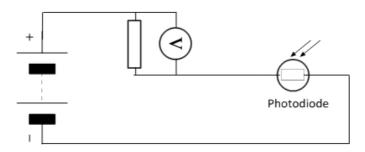
This kind of circuit can be used to test the transparency of various materials. A tube with a fixed diameter is placed directly over the top of the photodiode to prevent other light from reaching it. Various materials are placed one by one over the tube, and the photocurrent is calculated and recorded.
