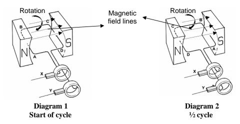
The coil is turned mechanically in a clockwise direction, i.e. AB starts moving upwards from the horizontal and CD starts moving downwards (as shown in Diagram 1).
