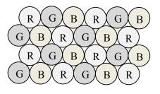
When an electron beam strikes a red phosphor dot it glows red; similarly the green and blue phosphor dots glow green and blue respectively when an electron beam strikes them. These electron beams are therefore called the red, blue and green beams.
