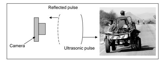
When you push the auto-focus button on the camera, it sends out a pulse of ultrasonic sound that travels to the object being photographed. Like an echo, the pulse reflects off the subject and returns to the camera.
