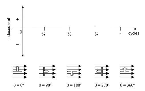
The group of arrows indicates the direction of the magnetic field and the block arrow indicates the direction of motion of **AB** of the coil. The angle  $\theta$  indicates the angle through which section **AB** has turned.
