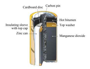
It is known scientifically as a Leclanché cell and commonly called a zinc-carbon cell. This is an example of a primary cell which is used in torches, toys and small appliances. There is a casing of zinc around the cell known as the **zinc can** which surrounds a chemical paste containing ammonium chloride and manganese dioxide. This paste is in contact with a central carbon electrode which runs the length of the cell.
