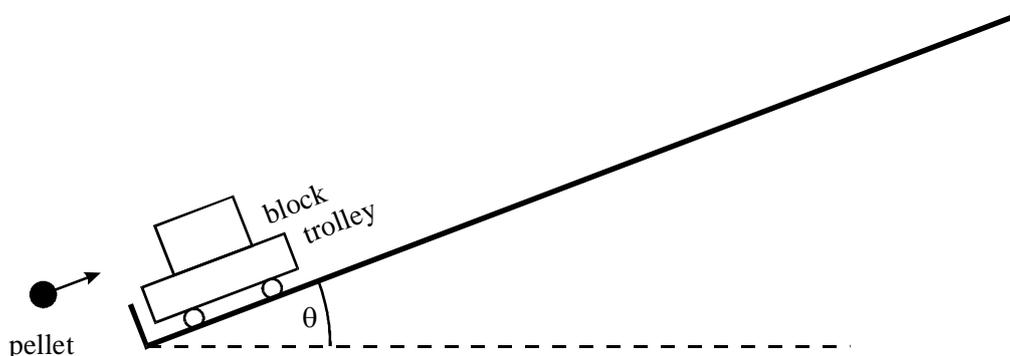
The pellet which is moving parallel to the track, strikes the block, embedding itself. The trolley and the block then move along the track, rising a vertical height,  $h$ .
