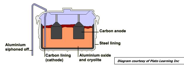
Diagram of an electrolytic cell used for the electrolysis of aluminium oxide
