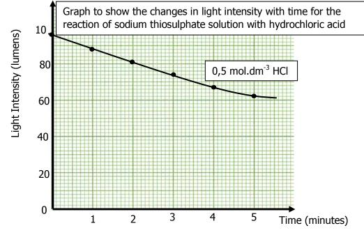
A graph representing the results of this experiment with 0,5 mol.dm<sup>-3</sup> HCl is shown below.
