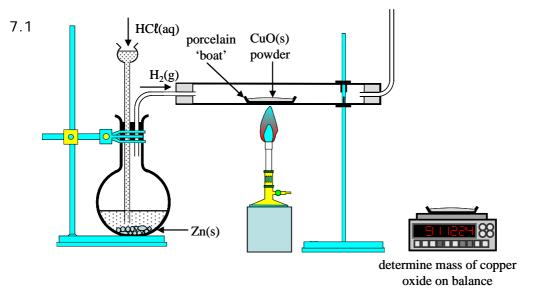
Copper oxide in the porcelain boat ✓ Boat and copper oxide placed inside the horizontal tube. ✓ Hydrogen passed from the hydrogen generator through the tube ✓ Burner beneath the boat containing the copper oxide ✓ (4)
